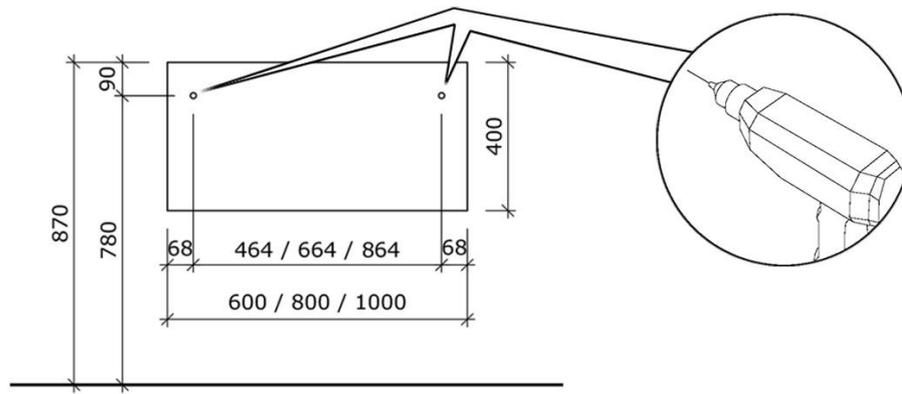
Measurements in mm
