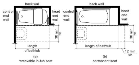
Clearance in front of bathtubs shall extend the length of the bathtub and shall be 30" wide minimum. A permanent seat at the head end of the bathtub or a removable in-tub seat shall be provided. Seats shall comply with 610.
