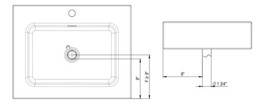
All **ORBIS** wall-mounted washbasins are ADA compliant. On Made to Measure orders, the dimension F has to be higher than 9".
