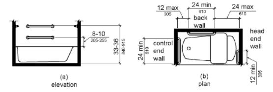
Grab bars for bathtubs shall comply with 609 and shall be provided in accordance with 607.4.1 or 607.4.2.
