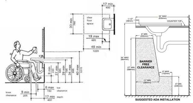
One key ADA requirement for wall-mounted lavatory washbasins is the maximum height of 34" from the finished floor (606.3). The required knee clearance (306.3) from the floor (up to 27" height) can be fulfilled with the Schmidlin wall-mount washbasins when installed on the correct height.
