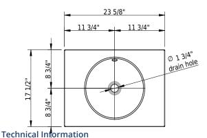
Bowl configurationsingleBowl depth5 1/2"Bowl sizeØ 14 1/8"Water depth to overflow3 5/8"Drain hole diameter1 3/4"
