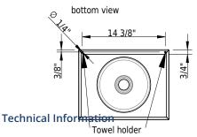
Bowl configurationsingleBowl depth4 3/8"Bowl sizeØ 9 3/8"Drain hole diameter1 3/4"
